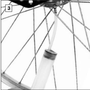
Remove the drain screw (3mm allen key) and refit the filling tube and syringe. Turn the wheel, so that the filling point is underneath the hub. Wait approx. 15mins with the wheel in this position, then use the syringe to draw out the old fluid. Remove the syringe and filling tube, use this to empty the fluid into the empty 50ml cleaning oil bottle.
