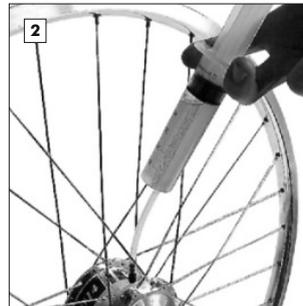
Draw the 25ml cleaning oil into the syringe, screw the filling tube into the drain screw hole and fill the cleaning oil into the hub. **After this, use the syringe to draw out a little air out into the syringe.** Remove the filling tube and refit the drain screw.
