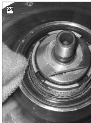
Remove the ring and the sprocket tool.
