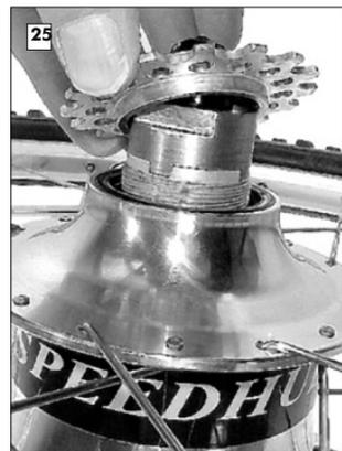
Replace the new/rotated sprocket (with undamaged seal surfaces) as shown in the Owners Manual.
