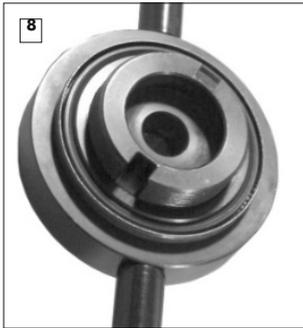
Place the new hub seal around the centering collar of the press tool.
