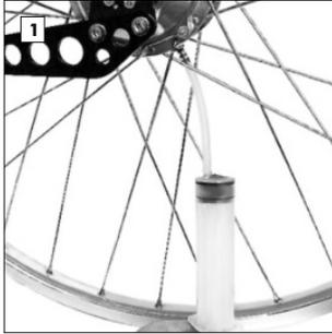
The removal procedure must start with the rinsing and draining of the oil from within the hub (see chapter "Oil change"). The drain screw must not be reused.
