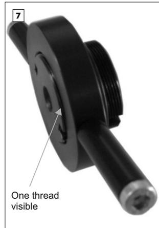
Prepare the hub seal press tool as shown in the picture.
