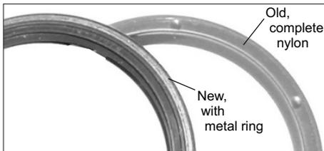
Check which type of hub seal is mounted within your hub. Hubs produced after Serial Number 25400 are equipped with the new hub seal. To be sure: The new hub seals have an outer metal ring and can therefore be replaced with the tools shown. The older types are completely formed from nylon, hubs needing these types of seals to be replaced, must be sent back to Rohloff Service department to be replaced.
