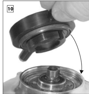
Place the press tool onto the hub with the new hub seal facing inwards.
