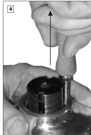
Remove the old hub seal by sharply pulling the removal tool upwards. If this doesn't remove the seal from the hub shell, then follow the method shown below.
