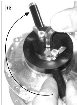
Turn the press tool clockwise as far as possible whilst holding the insert still with an 8mm allen key. The new hub seal will now be pressed firmly into the correct position.
