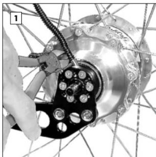
Remove the rear wheel. With good wire cutters, cut off the four cable ties that hold the concertina tubes over the hub cables.
