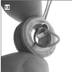
Next push the other end of the cable into the top hole of the cable pulley until both ends of the cable stick approx. the same length out of the other side.
