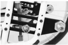
**Wheelbase extension via „grid mechanism with pulling operation“**
