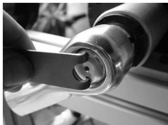
Fig. 6: Hold the gear shift button with the small wrench and tighten it with the 1.5mm hex bit.
