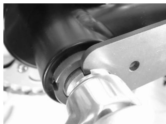
Fig. 8: Adjusting of gearing play. No preload!
