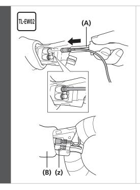
Open up the bracket cover and lift up the connector cover.
