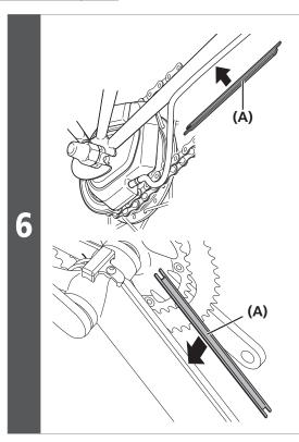
Install the electric wire cover/cord cover onto the frame.
