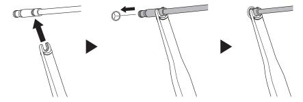
• When disconnecting the EW-SD300, the method below can also be used. Lift the TL-EW300 straight up as indicated in (A), or use the TL-EW300 as a lever as indicated in (B).
