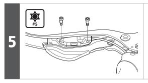
Return the switch unit to the setting position for the switch unit setting plate, and while pressing it by hand, operate the shifting switches [X/Y] once more and check that the switches turn on.
