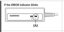
If the ERROR indicator blinks, the ambient temperature during charging may fall outside the operating temperature limits.
