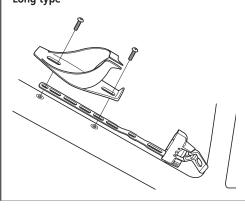
Use the bolts which are included with the bottle cage to secure the long type.
