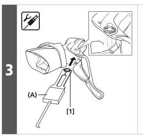
Use part [1] of the SHIMANO original tool to install the snap ring.
