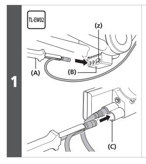
Connect the electric wire to the SC-S705 E-TUBE ports and junction [B].
