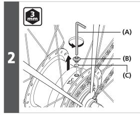
Remove the oil port bolt and O-ring.
