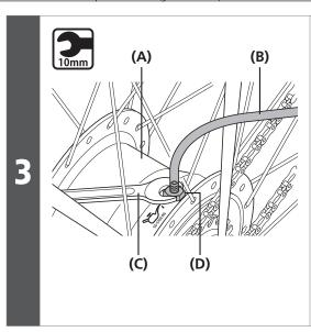
Attach the bleed nipple with tube attached to the hub shell.
