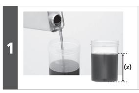
Fill the container with maintenance oil to a height of 95 mm.
