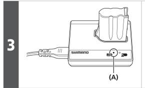
When the CHARGE indicator (orange) switches off, charging is complete.
