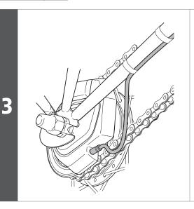
Temporarily secure the electric wire along the frame with tape, and connect it to junction [B].
