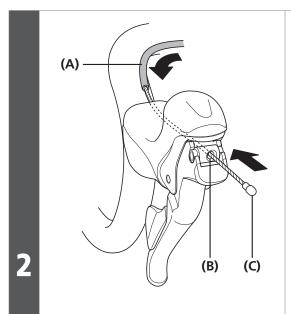
Pass the inner cable through from directly in front, set the inner cable drum into the cable hook, and then install the outer casing from the opposite side.
