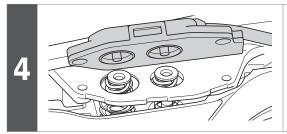
Make a gap between the switch unit and the setting plate and check that the end of the rubber on the switch unit is on the button.
