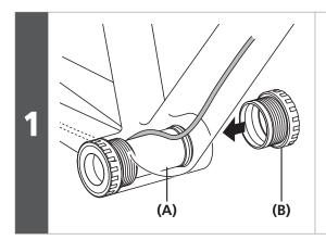
When installing the inner cover to the hanger, pass the electric wires for the motor unit and the built-in battery over the inner cover.
