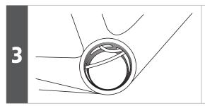
Make only the electric wires for the motor unit and the built-in battery visible inside the hanger; push unnecessary protruding components such as the wire holder into the frame.
