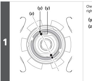
Check that the two • marks (red) on the right side of the hub body are aligned.
