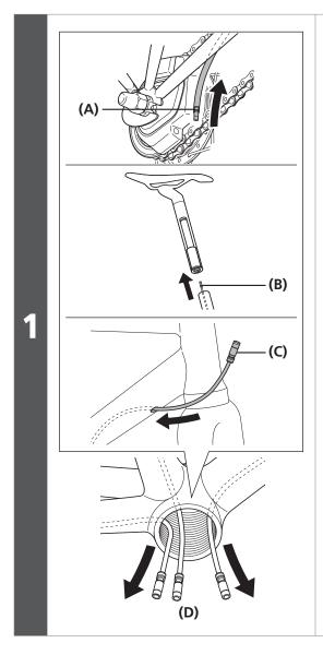
First, insert the electric wire for each of SC-S705, the battery mount, and the motor unit through the hole in the frame to the bottom bracket shell.
