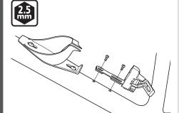
Use the included M4 screws to secure the short type.
