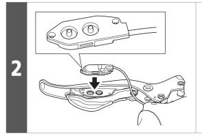
Place the switch unit onto the mounting surface of the setting plate.
