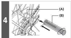
With the piston of the syringe pushed fully in, firmly connect the syringe to the tube.
