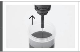
Remove the internal unit from the oil.
