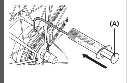
Push the piston to inject the new oil into the inside of the hub.
