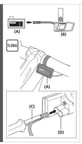
Connect the electric wire of the shifting switch to the system information display (SC-S705) using TL-EW02.
