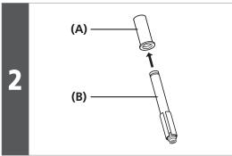
Insert the lithium ion battery (built-in type) into the seat post collar from the bottom of the seat post.
