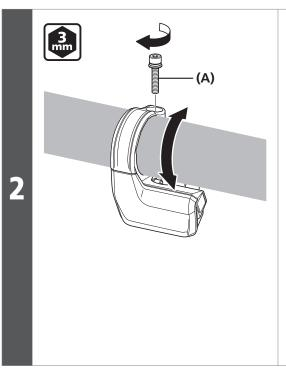
Adjust the angle of the system information display so that it is easy to see, and then use a 3 mm hexagon wrench to tighten the clamp bolt.
