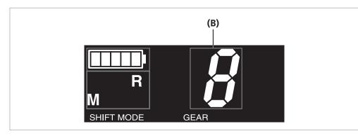
(B) Gear position/Adjustment level
