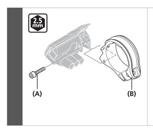
Remove the case mounting bolt with a 2.5 mm hexagon wrench and replace the clamp band.
