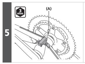
Once the electric wires have been routed, secure junction [B] underneath the bottom bracket shell.
