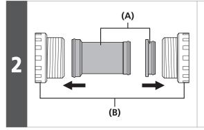
Install the inner cover to the bottom bracket adapter.
