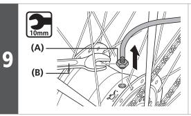
While being careful that the tube does not come off the syringe, remove the bleed nipple.
