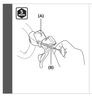
Pull back the bracket cover from the front and use a 5 mm hexagon wrench to tighten the fixing nut.
