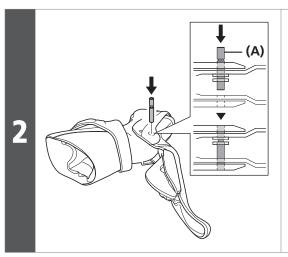
Align with the hole in the axle, and then press-fit the lever axle.
