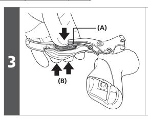
Press the switch unit by hand so that the switch springs go into the grooves in the buttons, and then push the shifting switches [X/Y] in as far as they will go.
