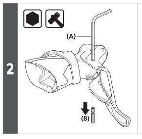
Insert a hexagon wrench or a similar tool into the hole in the lever axle, and then tap it with a soft face mallet to push out the lever axle.
