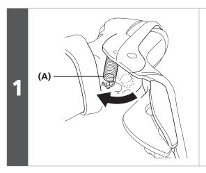
Assemble the bracket body and the lever body, and then attach the return spring.
