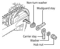
When installing the hub to the frame, the chain guard may come off, so check that the chain guard is securely installed.
