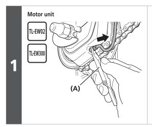
Remove the electric wire on the motor unit side.
