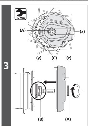
Install the motor unit to the hub so that the • mark (x) on the motor unit is aligned with the • mark (y) on the hub lock spacer.
