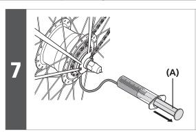
Pull the piston out slowly to draw out the oil inside the hub shell.
