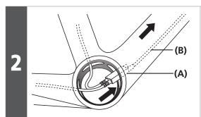
Install the electric wire for the system information display and junction [B] inside the down tube.
