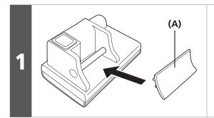
Install the rubber spacer to the system information display.
