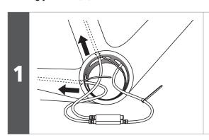
Pass the electric wires for the motor unit and the built-in battery through the chainstay and the seat tube, respectively.
