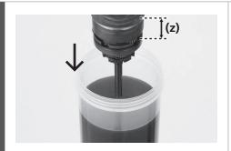
Immerse the internal unit in the oil from the left side until the oil reaches up to ring gear unit 1, as shown in the illustration.
