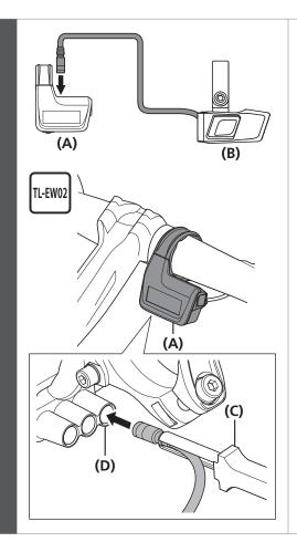
Connect the electric wire of the shifting switch to the system information display (SC-MT800) using TL-EW02.
