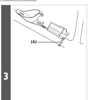
Tighten the bolt of the bottle cage to secure the battery mount.
