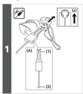
Use the SHIMANO original tool which is sold separately to remove the snap ring.
