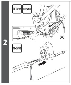
Connect the electric wires to the motor unit and the battery mount.
