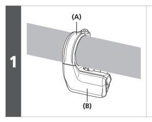
Insert the clamp band of the system information display into the handlebar.
