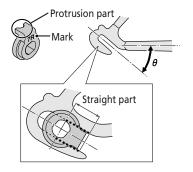
Install the non-turn washer so that the protrusion fits securely in the dropout groove at the front and back sides of the hub axle.
