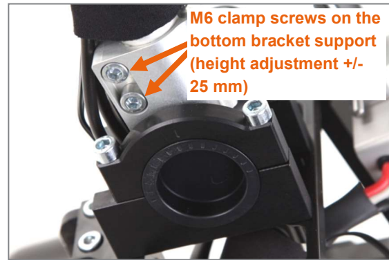
Figure 15: M6 clamp screws for adjusting the height of the bottom bracket position
