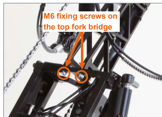
Figure 12: M6 fixing screws on the top fork bridge
