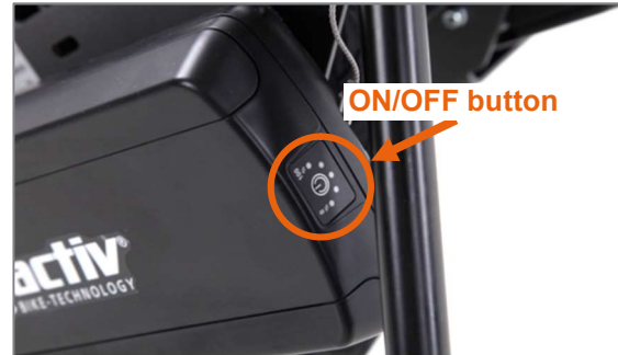
Figure 37: On and off button on the rechargeable battery
