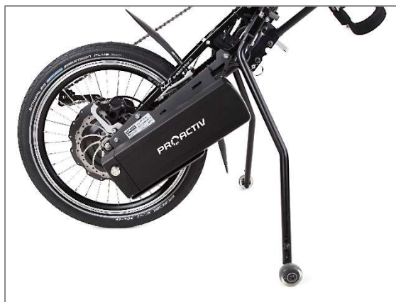
Figure 7: Parking stand in the active position
