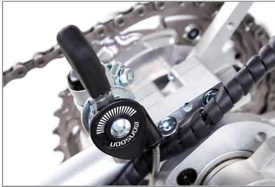
Figure 29: Parking brake via locking lever
