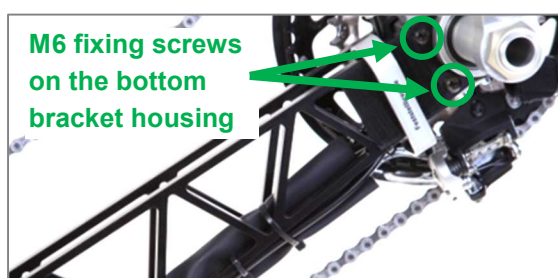
Figure 13: M6 fixing screws on the bottom bracket housing
