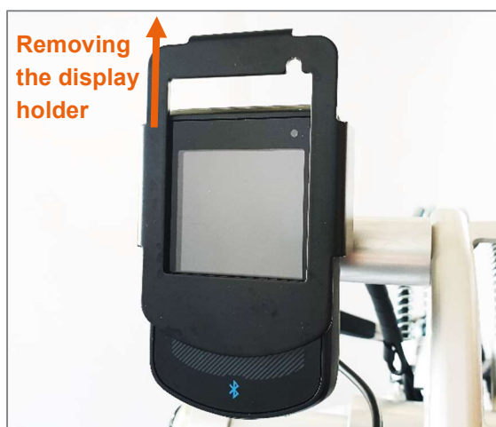
Figure 40: removing the display holder
