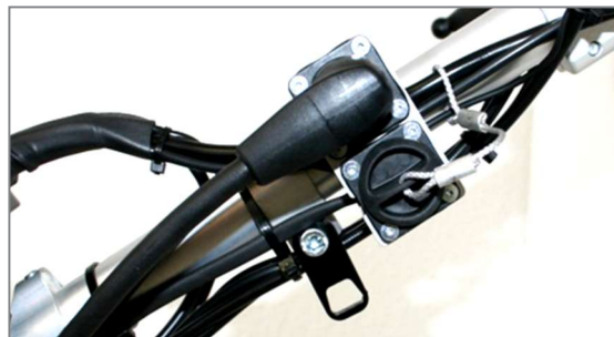
Figure 31: Change-over device on the steering column
