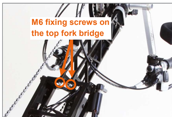
Figure 12: M6 fixing screws on the top fork bridge
