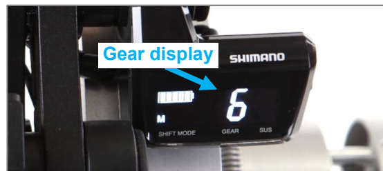
Figure 21: Displaying the current gear on the display
