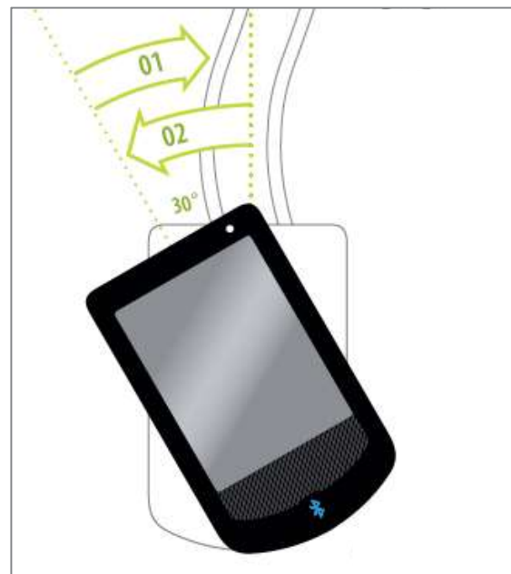
Figure 38: Attaching and removing the display
