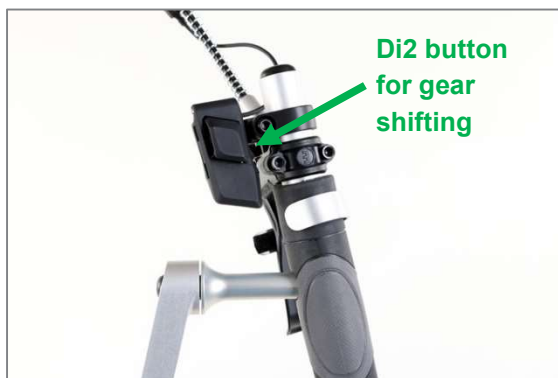
Figure 19: Operation via the button
