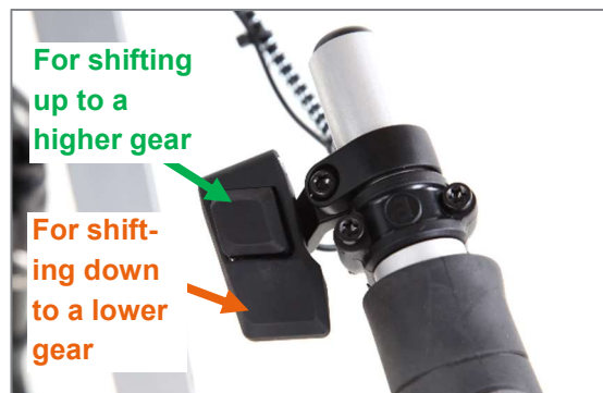
Figure 20: Buttons for shifting up and down
