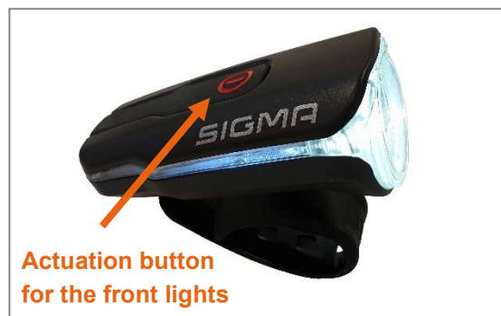
Figure 41: Actuation button for the front lights
