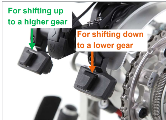
Figure 22: Chin operation via buttons
