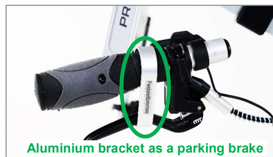
Figure 28: Aluminium bracket as a parking brake
