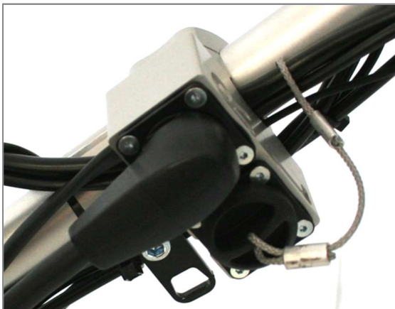
Figure 34: Right rechargeable battery connected; magnetic connector in "R" socket
