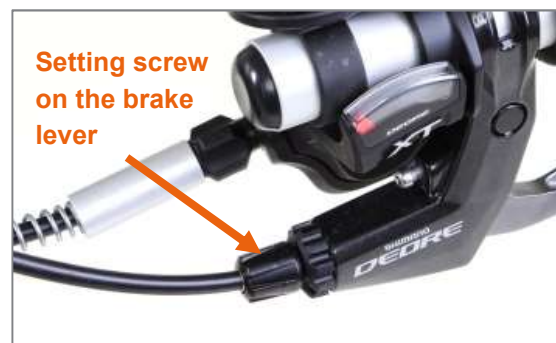
Figure 27: Setting screw on the brake lever
