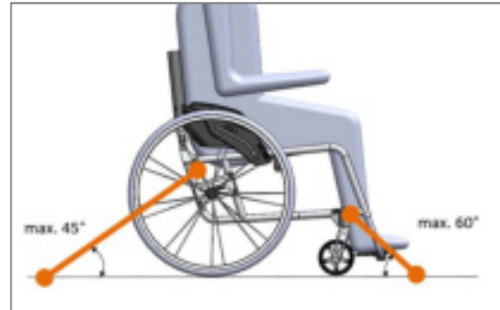
Figure 186: Run of the retractors at the front and rear with maximum tensioning angle and connecting points (view from the side)
