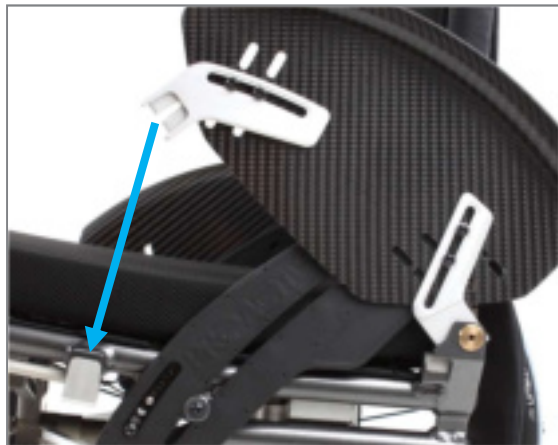
Figure 55: Rear side section mount mounted on back jointed shaft (view without drive wheel)
