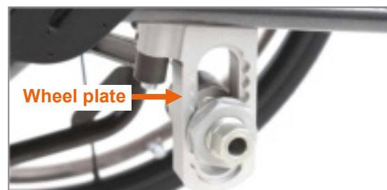
Figure 6: Wheel plate for rear seat height adjustment (drive wheel removed)
