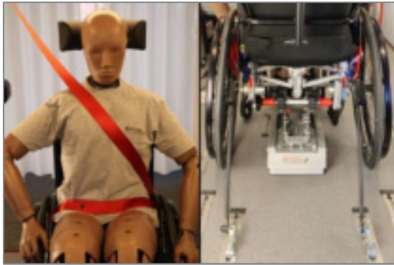
Figure 195: Occupant belt restraints should make full contact with the shoulder, chest and pelvis and pelvic belts should be positioned low on the pelvis near the thigh-abdominal junction
