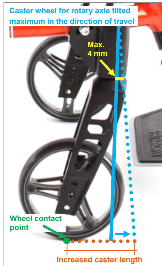
Figure 95: Increased caster length via the inclination of the caster wheel axle
