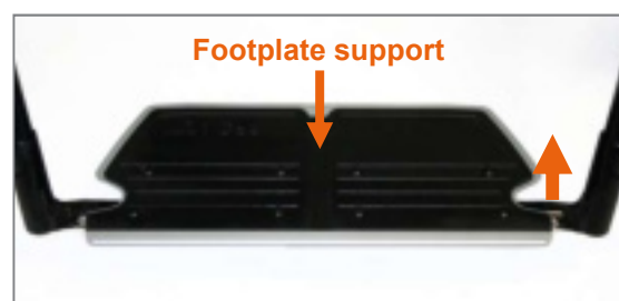
Figure 111: For folding up to one side, lift the footrest up in the direction of travel on the left side (product view from the front)
