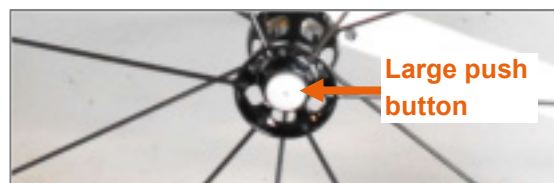
Figure 69: Quick-release axle with operation support, large push button
