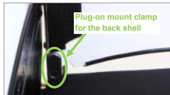
Figure 48: Plug-on mount clamp for the back shell (view from front)
