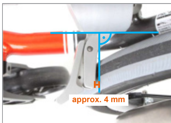
Figure 161: Brake element after correct positioning of the integral brake
