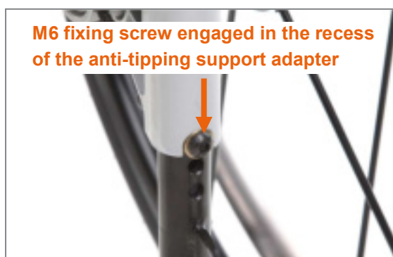
Figure 133: Anti-tipping support engaged correctly
