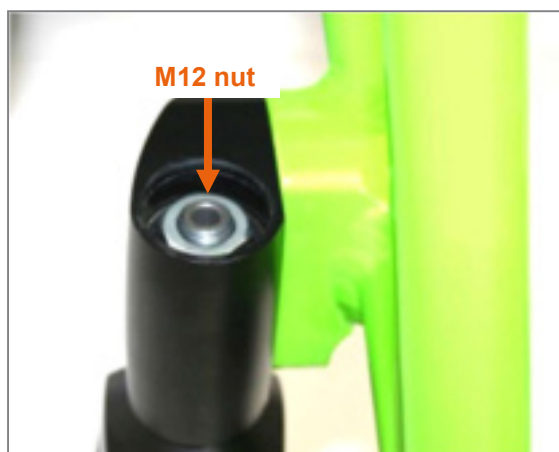
Figure 97: Aluminium cap removed and M12 nut visible
