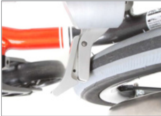
Figure 156: Brake element resting on the tyre
