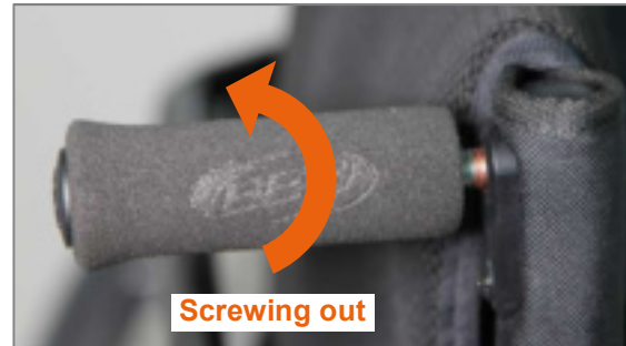
Figure 165: Screw the push handle horizontally out of the back tube
