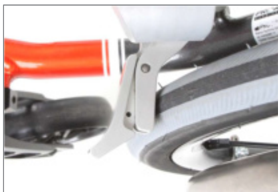
Figure 160: Brake element resting on the tyre
