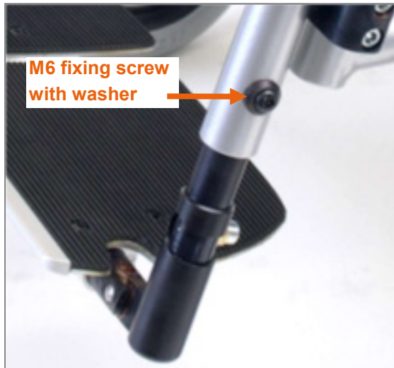
Figure 128: M6 fixing screw with washer to adjust the lower leg length
