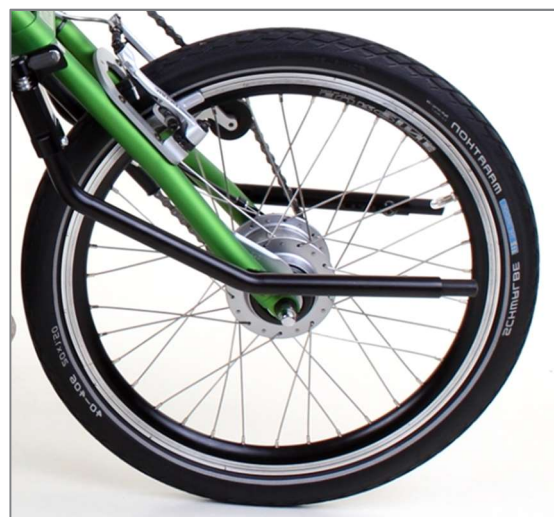
Figure 8: Parking stand in the passive position
