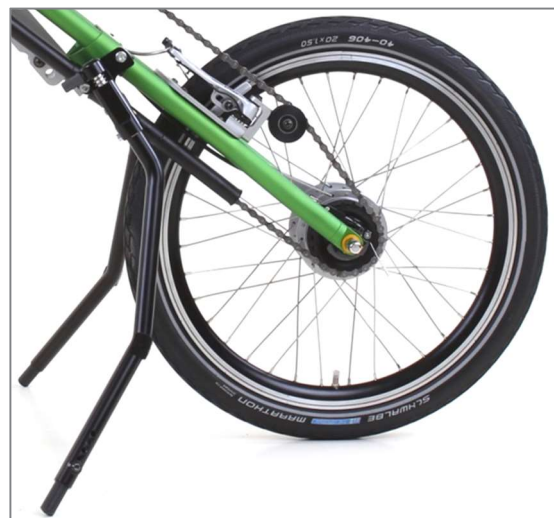
Figure 7: Parking stand in the active position
