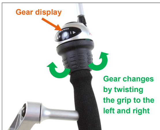
Figure 17: Shifting using the grip shift for the Shimano Nexus hub gear
