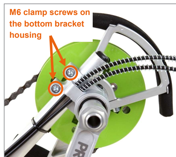
Figure 13: M6 clamp screws on the bottom bracket housing for the height adjustment of the bottom bracket position and the replacement of the bottom bracket support
