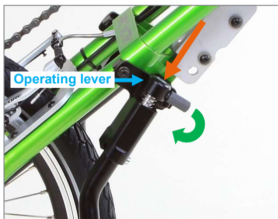
Figure 6: Press down and turn the operating lever
