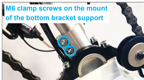
Figure 14: M6 clamp screws on the mount of the bottom bracket support for the height adjustment of the bottom bracket position and the replacement of the bottom bracket support
