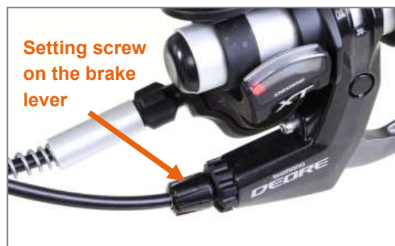
Figure 22: Setting screw on the brake lever
