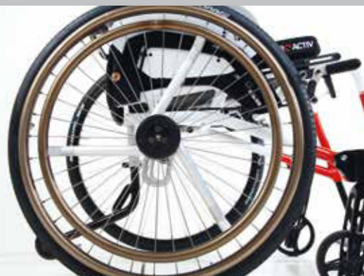
Frame inner tubes, diagonal strut and long wheel plate inlet as heavy duty equipment
