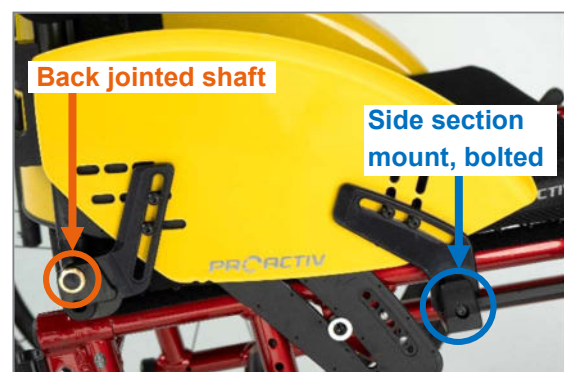
Figure 28: Clothing guard mounted on product (view without drive wheel)
