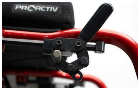
Figure 100: Knee lever brake system equipped with brake lever at 20°
