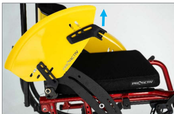
Figure 30: Clothing guard pulled from the "side section mount, bolted" at the front (view without drive wheel)
