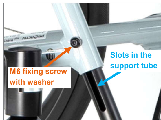
Figure 77: M6 fixing screw with washer and slot in footrest support tube for adjusting the lower leg length
