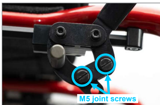
Figure 105: M5 joint screws for setting the actuating force of the brake lever
