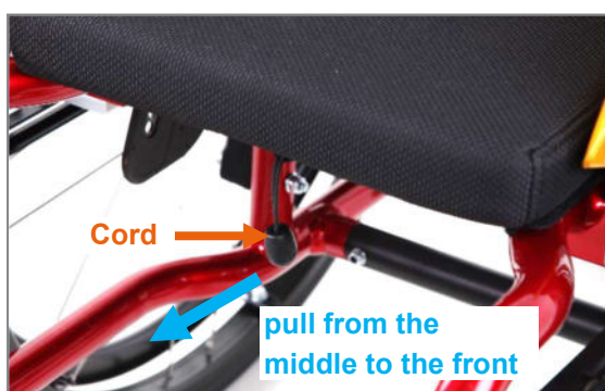
Figure 17: Cord for operating the locking pin and thus for adjusting the angle of the backrest
