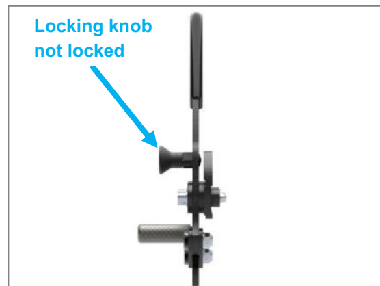
Figure 108: Locking knob pulled out of lock and turned 90° (view from the front)
