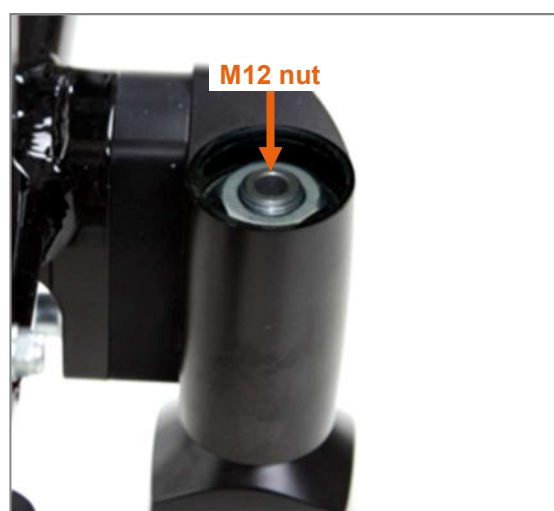
Figure 69: Aluminium cap removed and M12 nut visible
