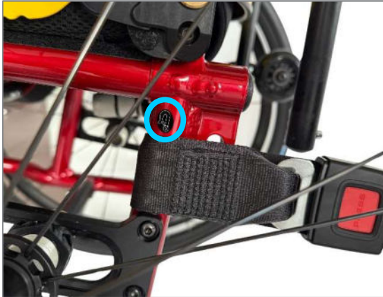
Figure 141: Symbol for rear fastening and wheelchair loop at the rear
