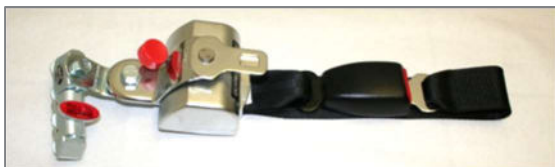
Figure 132: Front retractor "semi-automatic" with buckle and belt link
