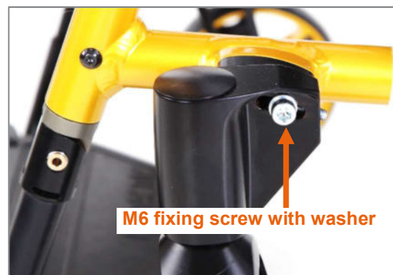
Figure 74: M6 fixing screw on the frame outer side
