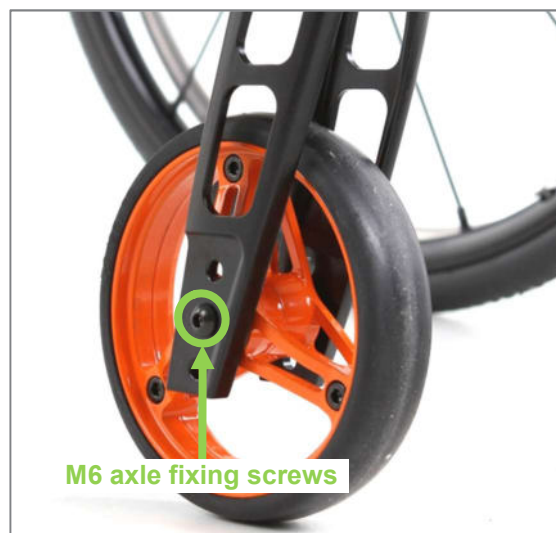
Figure 59: M6 axle fixing screw of caster wheel axle (view from outer side of product)
