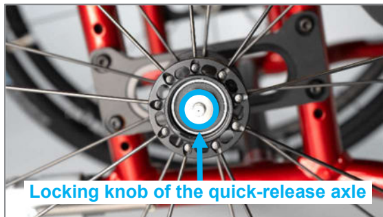
Figure 43: Locking knob of the quick-release axle in the middle of the wheel axle
