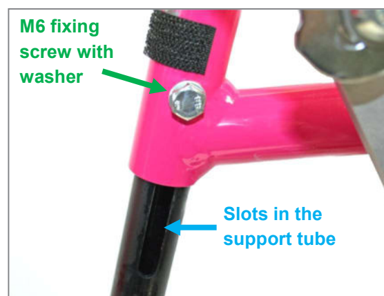
Figure 90: M6 fixing screw with washer and slot in footrest support tube for adjusting the lower leg length
