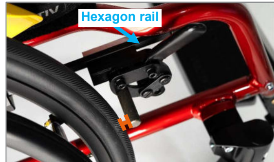
Figure 104: Distance between the brake pin and tyre of approx. 3 to max. 4 mm with the brake opened
