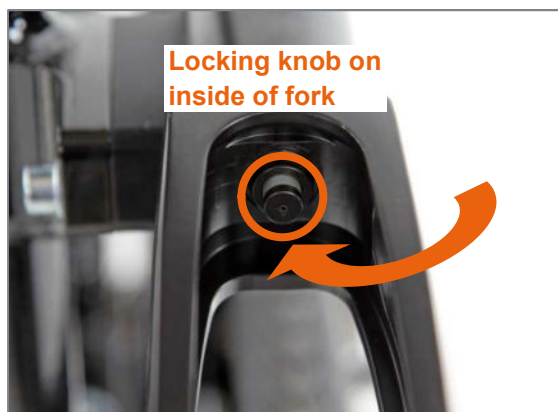
Figure 70: Caster fork with quick-release axle and locking knob
