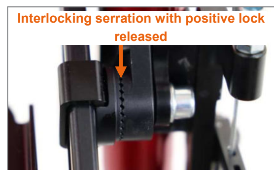
Figure 93: Serration on foot bracket clamps, positive locking undone
