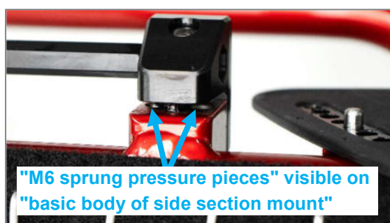
Figure 39: Front side of the sprung pressure pieces visible (view from top)
