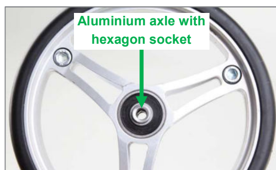
Figure 60: Caster wheel with aluminium hexagon socket
