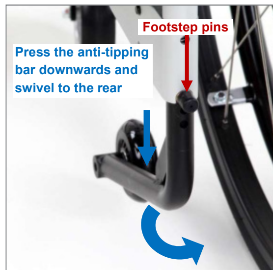
Figure 121: Moving the anti-tipping support to operating position (view from the rear)
