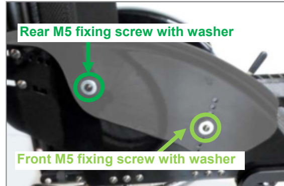
Figure 35: Side panel with bolt-on clothing guard and M5 fixing screws (shown without the drive wheel)
