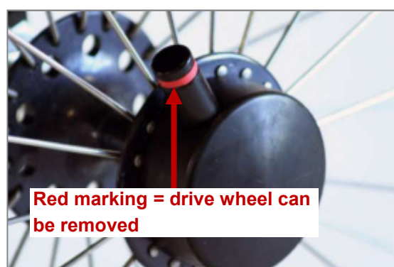
Figure 58: Tetra Clip with opened quick release axle, drive wheel can be removed
