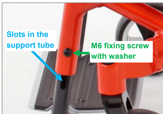
Figure 102: M6 fixing screw with washer and slot in footrest support tube for adjusting the lower leg length
