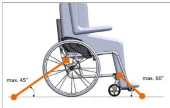
Figure 186: Run of the retractors at the front and rear with maximum tensioning angle and connecting points (view from the side)
