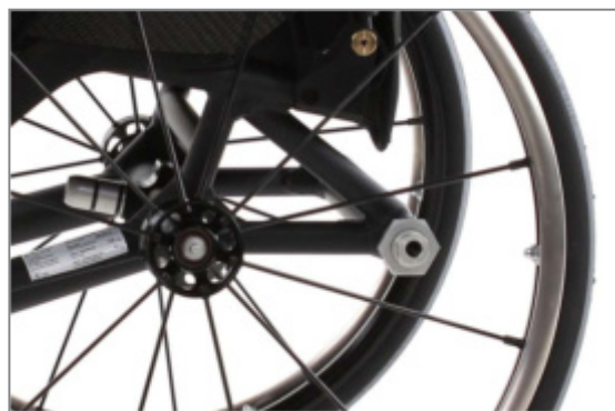
Figure 69: Wheelbase extension welded in place (SPEEDY F2 oversized)
