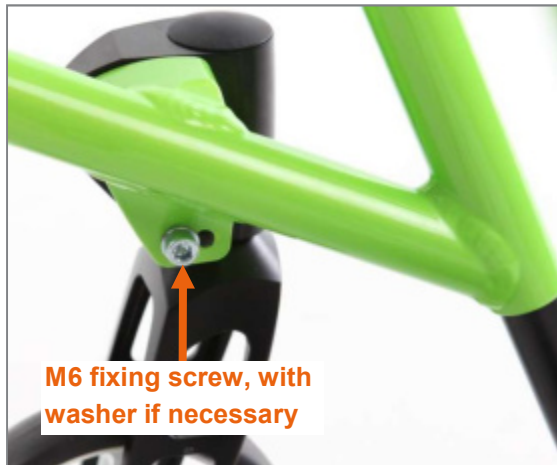
Figure 98: M6 fixing screw on frame inner side, washer fitted with G-shape frames but not V-shape frames
