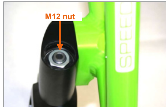
Figure 92: Aluminium cap removed and M12 nut visible
