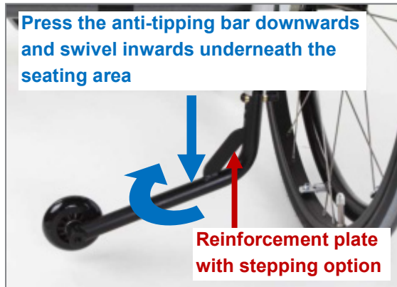
Figure 123: Moving the anti-tipping support to passive position (view from the rear)
