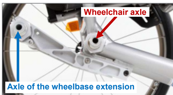
Figure 77: Wheelchair axle and wheelbase extension axle (view from outer side of product without drive wheel)
