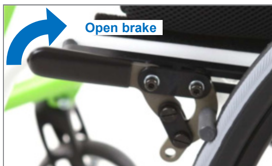
Figure 139: Brake closed; opening done by pulling the brake lever up and rearwards
