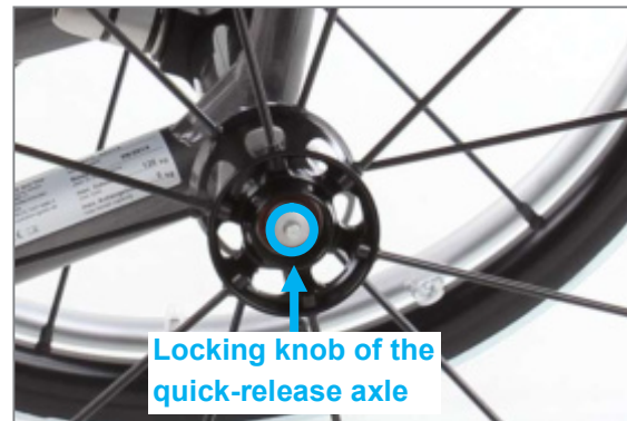
Figure 54: Locking knob of the quick-release axle in the middle of the wheel axle
