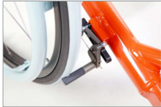
Figure 147: Brake closed, brake pin presses into the tyre by approx. 4 mm
