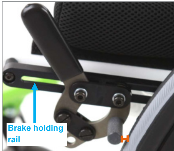
Figure 141: Distance between the brake pin and tyre of approx. 3 to max. 4 mm with the brake opened
