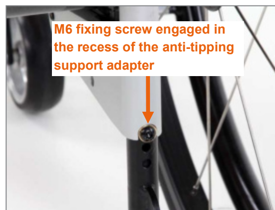
Figure 122: Anti-tipping support engaged correctly
