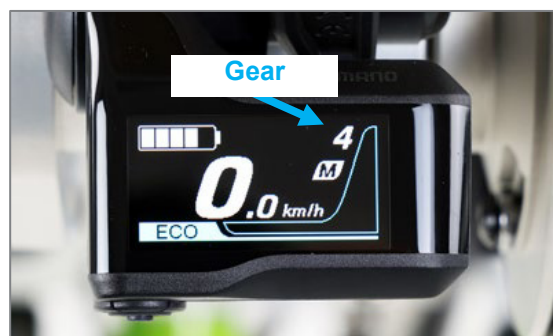
Figure 26: Displaying the current gear on the display
