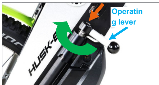
Figure 6: Press down and turn the operating lever
