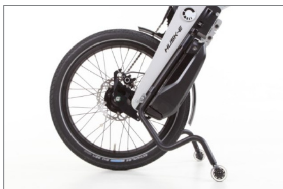
Figure 7: Parking stand in the active position
