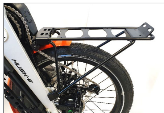
Figure 48: Luggage rack installed
