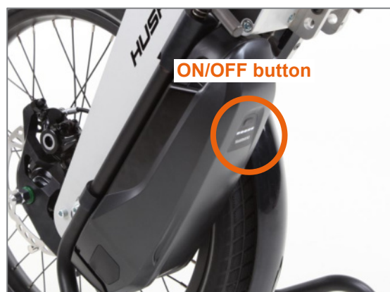
Figure 38: Switching the rechargeable battery on and off
