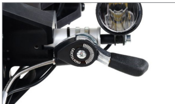
Figure 29: Parking brake via locking lever
