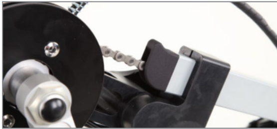
Figure 19: Plastic chain guides in rectangular tube
