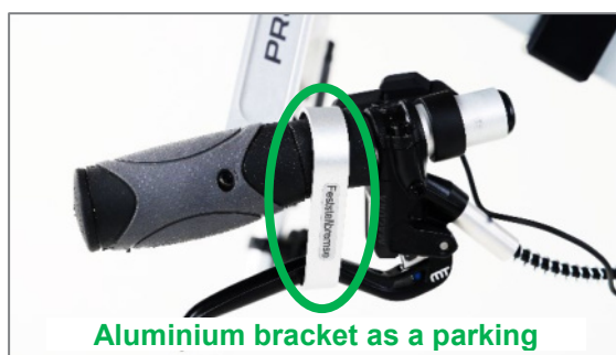
Figure 30: Aluminium bracket as a parking brake
