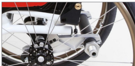
Figure 1: Removable wheelbase extension
