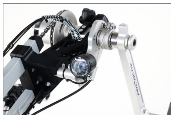
Figure 42: Front lights of the LED light set
