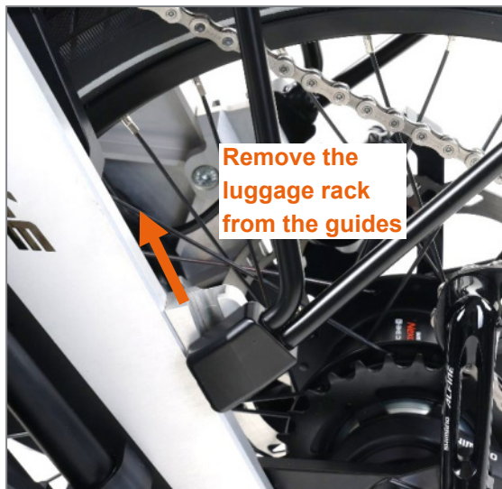
Figure 45: Removing the luggage rack from the guides
