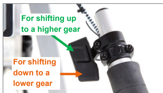
Figure 25: Buttons for shifting up and down
