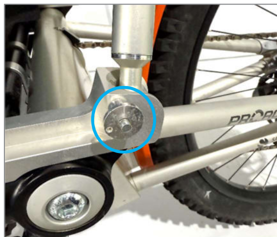
Figure 51: Quick-pin for the backrest on the joint slide (left)
