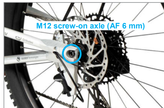
Figure 69: Screw-on axle of the drive wheel
