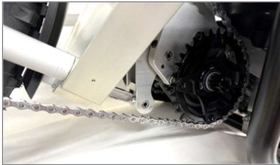
Figure 85: Deflector of the swing arm with coupling rod and chainring of the motor
