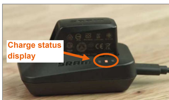
Figure 18: Rechargeable battery in the charger with display of the charge status
