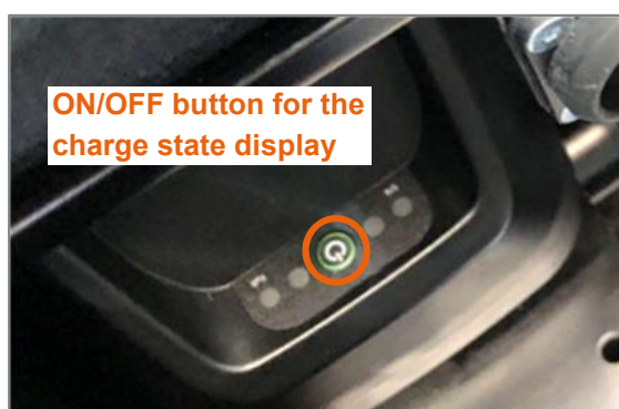
Figure 31: ON/OFF button for the charge state display
