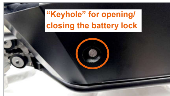
Figure 28: Keyhole for the battery accessible from the outside through the opening on the side guard
