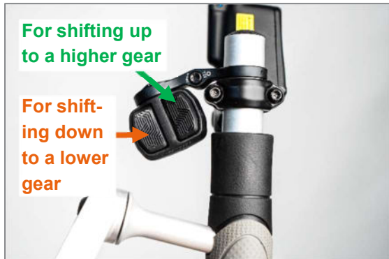
Figure 13: Button for shifting the SRAM gearshift up and down
