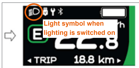
Figure 47: Indication on the display when the lighting is switched on
