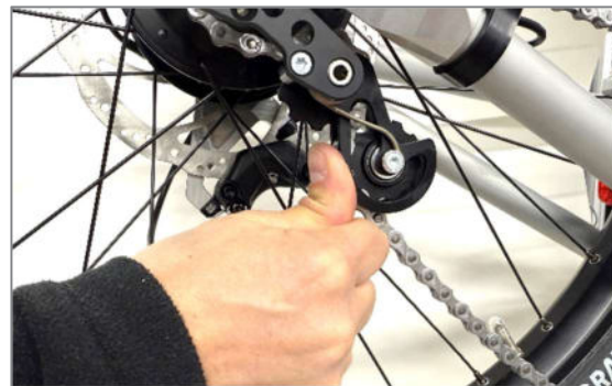
Figure 65: Relieving the chain tensioner
