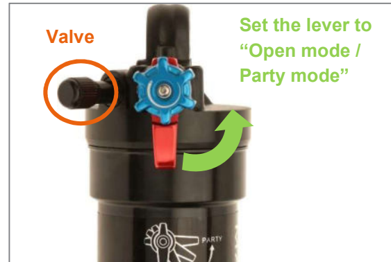
Figure 40: "Open mode / Party mode" lever position for Manitou Mara Inline dampers
