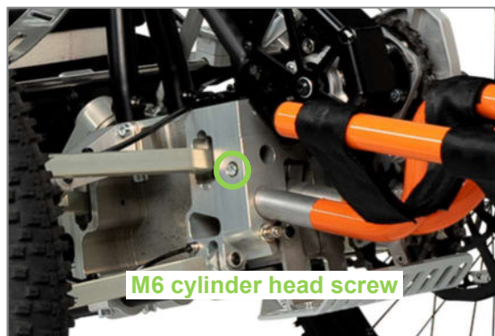
Figure 80: M6 cylinder head screw on the connection tunnel for removing the leg rest
