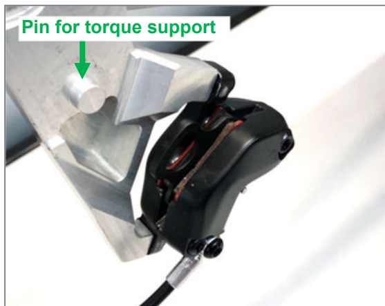
Figure 67: Left dropout with Rohloff hub
