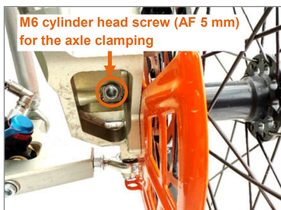
Figure 58: Axle clamping on the wheel carrier (view on the right running wheel)
