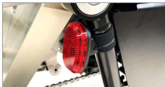
Figure 46: Rear lighting via drive system
