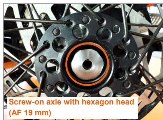
Figure 60: Wheel hub with screw-on axle
