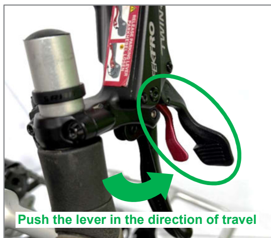
Figure 21: Parking brake activated
