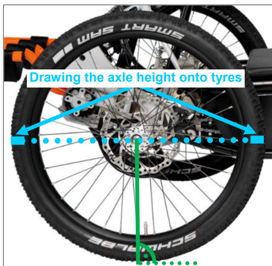
Figure 71: Drawing the axle height on the front and back of both tyres of the running wheels
