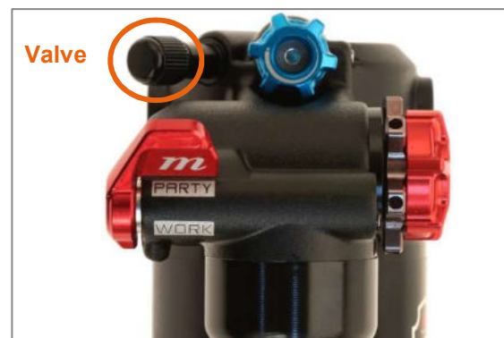
Figure 41: "Open mode / Party mode" lever position for Manitou Mara Pro dampers
