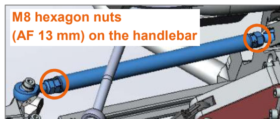
Figure 74: M8 hexagon nuts on the lower handlebars on the right and left
