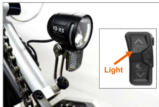
Figure 45: Front lighting via drive system
