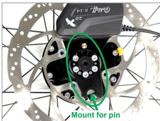
Figure 68: Torque absorption with Rohloff gearshift on the drive wheel (view on the inside of the wheel)
