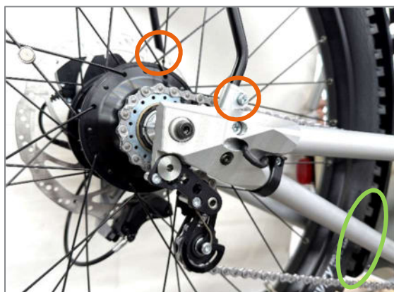
Figure 82: Position of the M5 cylinder head screws for fastening the mudguard
