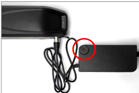
Figure 36: Rechargeable battery is being charged – LED is illuminated red
