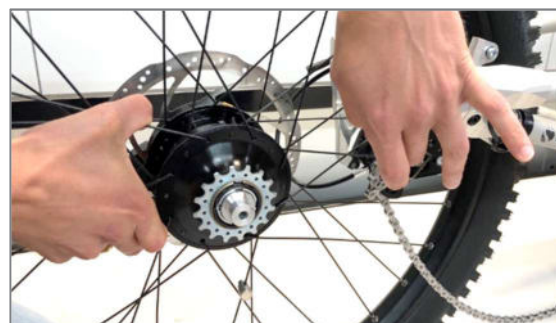
Figure 66: Taking the chain off of the sprockets
