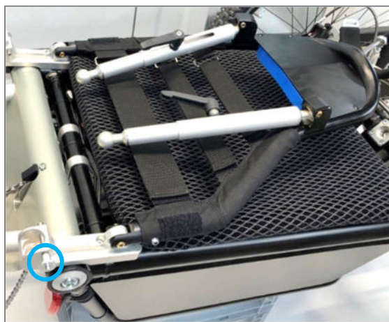
Figure 53: Backrest folded down and quick-pins re-inserted
