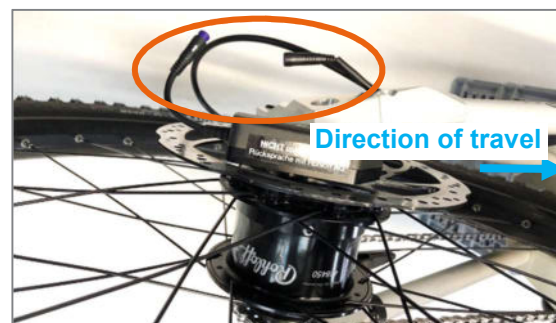
Figure 64: Released plug connection (view from the top)
