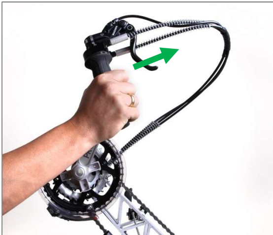
Figure 11: Correct hold of the handle for the Rohloff hub gear
