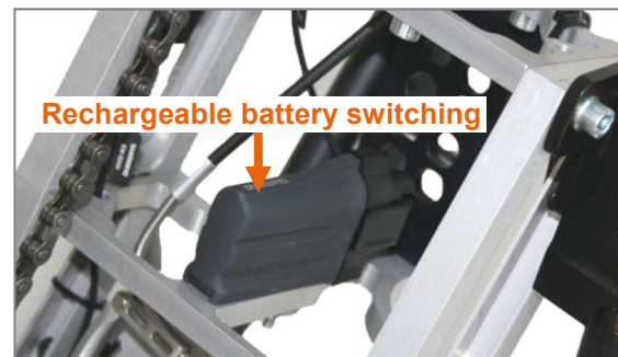
Figure 20: Alfine Di2 electronic gearshift battery
