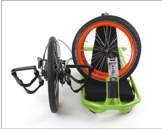
Figure 67: Pack size: Chassis and drive unit separated and running wheels removed
