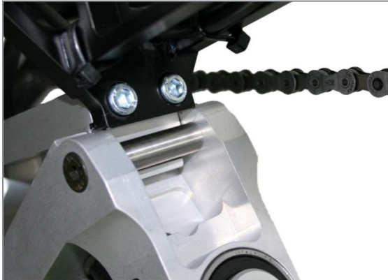
Figure 59: Insertion Maul of the drive unit slips under the insertion shaft on the chassis
