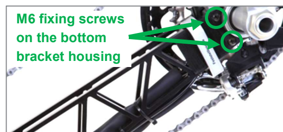
Figure 6: M6 fixing screws on the bottom bracket housing
