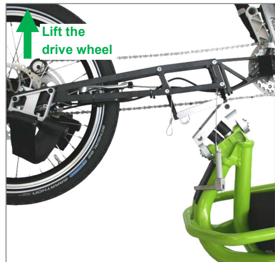
Figure 66: Lifting the drive wheel
