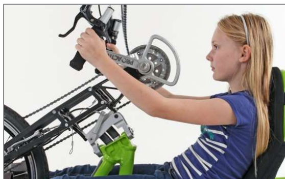
Figure 3: Elbows are not stretched completely
