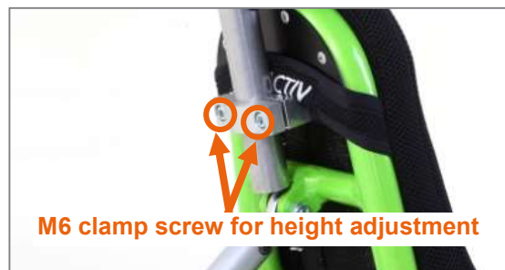
Figure 39: Height adjustment of the neck rest via two M6 clamp screws on the neck rest holding tube
