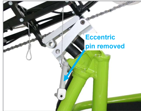
Figure 65: Eccentric pin removed from the adapter plate, chassis lowered to the ground
