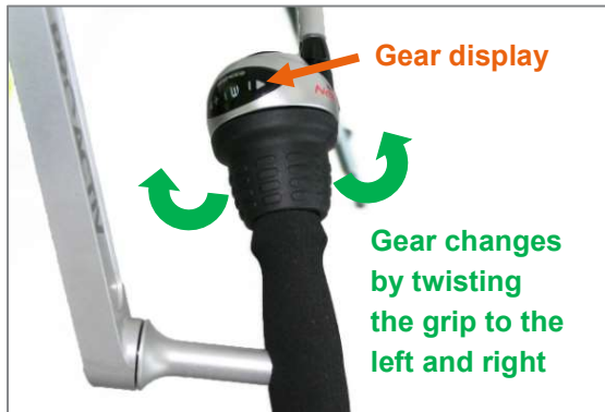
Figure 17: Shifting using the grip shift for the Shimano Nexus hub gear
