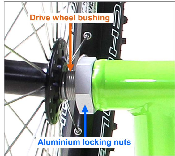
Figure 50: Drive wheel bushing and aluminium locking nut (rear view)
