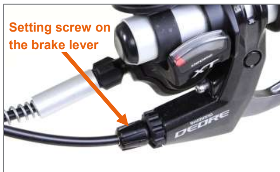
Figure 28: Setting screw on the brake lever
