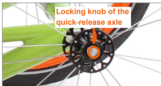
Figure 46: Locking knob of the quick-release axle in the middle of the wheel axle
