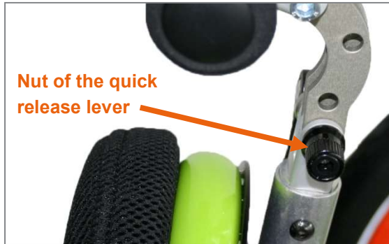
Figure 42: Nut of the quick release lever
