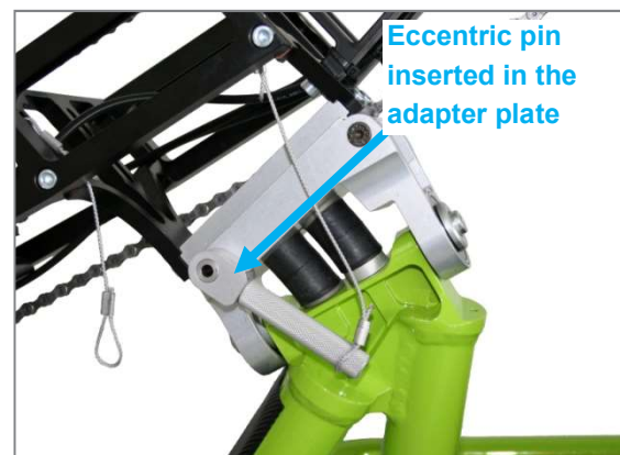
Figure 62: Eccentric pin inserted
