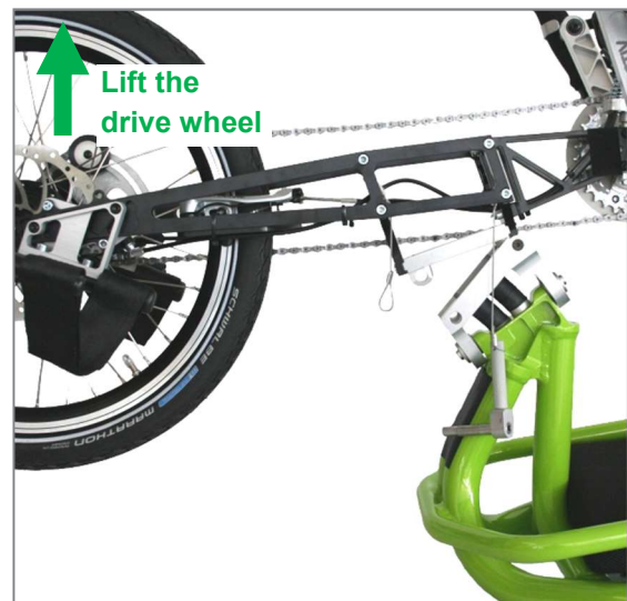
Figure 58: Lifting the drive wheel
