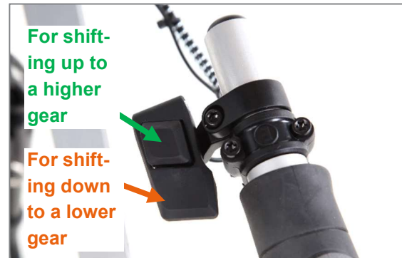
Figure 18: Buttons for shifting up and down
