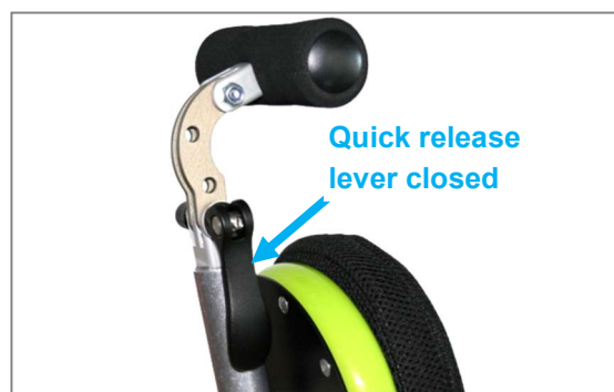
Figure 40: Quick release lever closed
