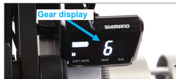
Figure 19: Displaying the current gear on the display
