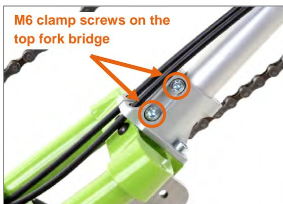
Figure 13: M6 clamp screws on the top fork bridge for replacing the pedal bearing support
