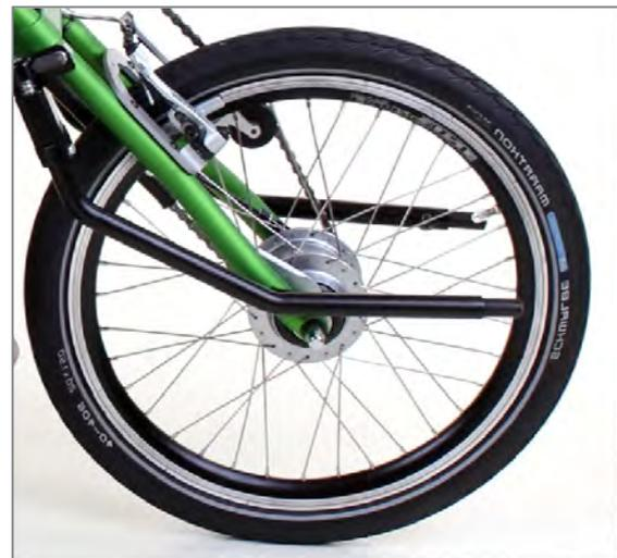
Figure 5: Parking stand in the passive position
