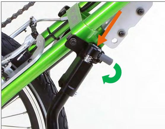
Figure 3: Press down and turn the operating lever
