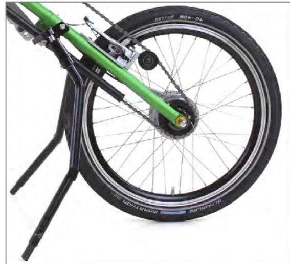
Figure 4: Parking stand in the active position
