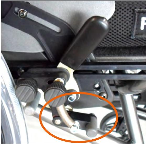
Figure 1: Anti-roll back device
